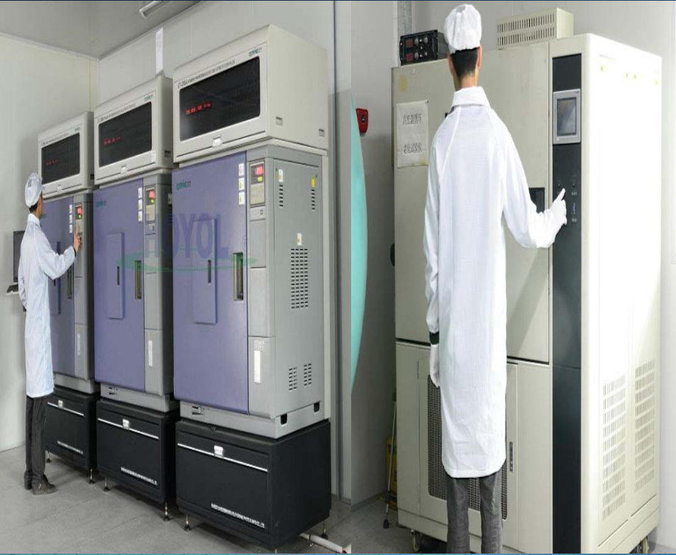
LED & LED module aging test system
